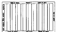
7600M Hydrodynamic Vane Grate Approx. 220 sq. in. open area "DUMP NO WASTE DRAINS TO RIVER"
